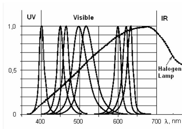
Fig. 1. The normalized spectra of the halogen lamp and the standard LED set
