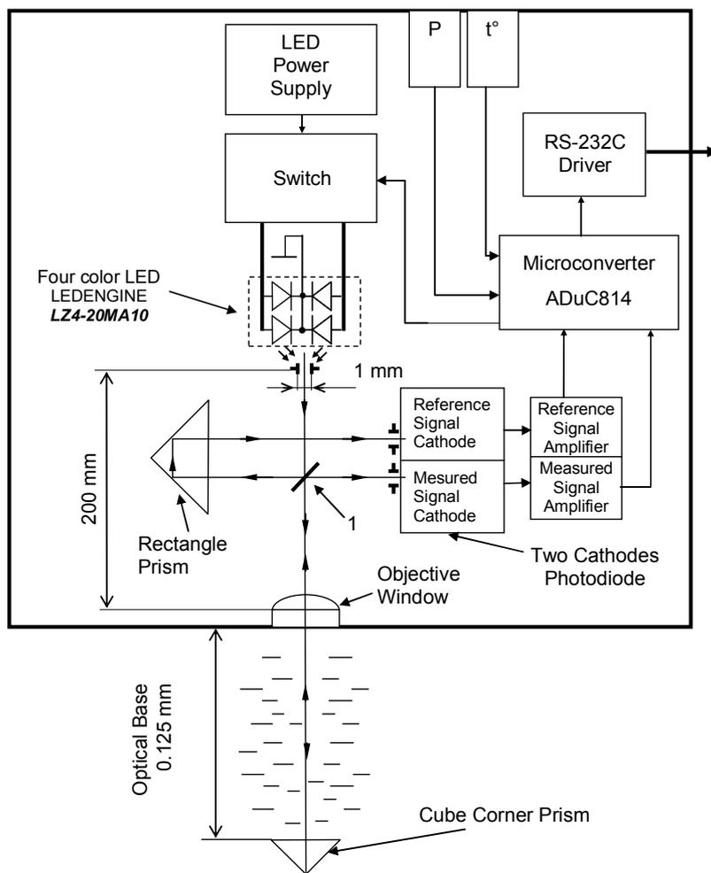
Fig. 3. The spectral attenuation meter structure scheme
