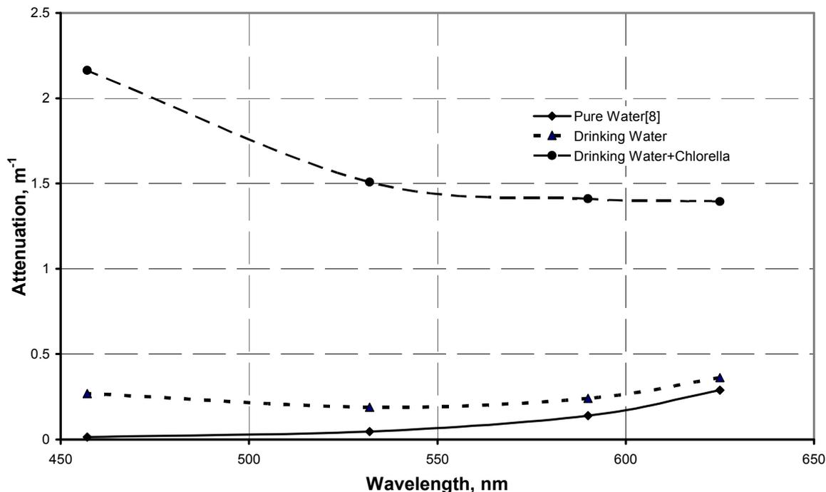
Fig. 4. An example of spectral measurements of BAC
