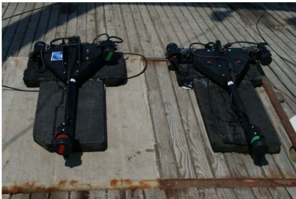
Figure 3 Free-fall optical profilers (NATO and JRC) deployed during the cruises. 2 Inherent Optical Properties (IOP)
